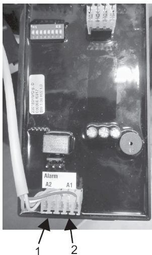
Fig. 4: Cable connection at the control unit
