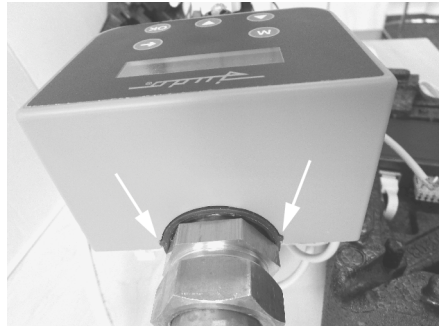
Fig. 11: Lock into place rear wall of electronic housing
