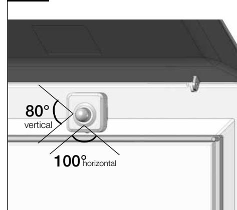
**6.4 Installation of humidity sensor ELS-VF.. (optional)**
